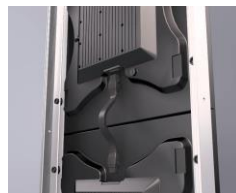
2. Connect Power&Signal 2 in 1 cable ;
